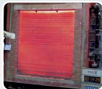
AFTER 3 hrs FIRE TESTING
